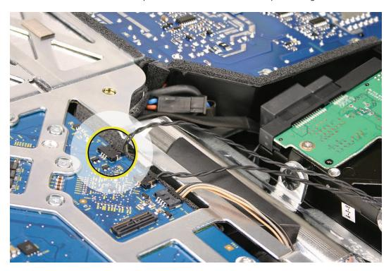
2. Push HARD and toward the logic board on the black plastic clip at the top of the hard drive to release it from the chassis.
